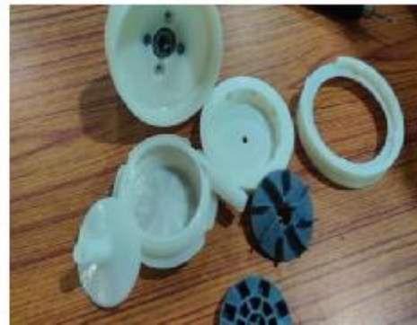
Fig.1.20: Surface roughness less than 3 micros achieved in 3D printed Prototype – with ABS material and post processing techniques.
