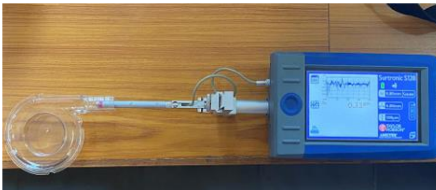
1.6b: Ra=0.33 for Injection Moulded Pump
