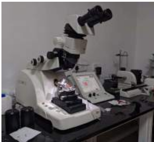
Fig-2 Microtomy of a sample for making thin section
