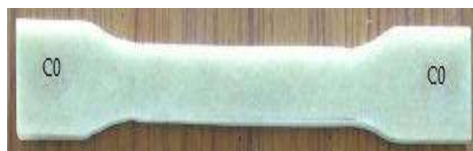
Fig.3.1. Specimen for Tension test (C0)
