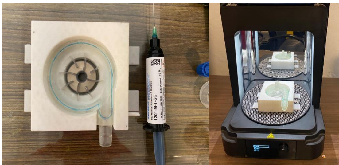
Glue added to clear 3D printed pump and cured in UV chamber
