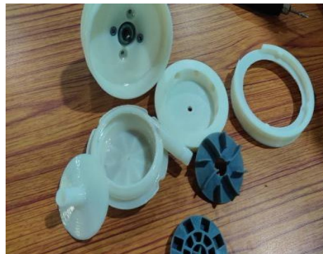
Surface roughness less than 3 micros achieved in 3D printed Prototype – with ABS material and post processing techniques.
