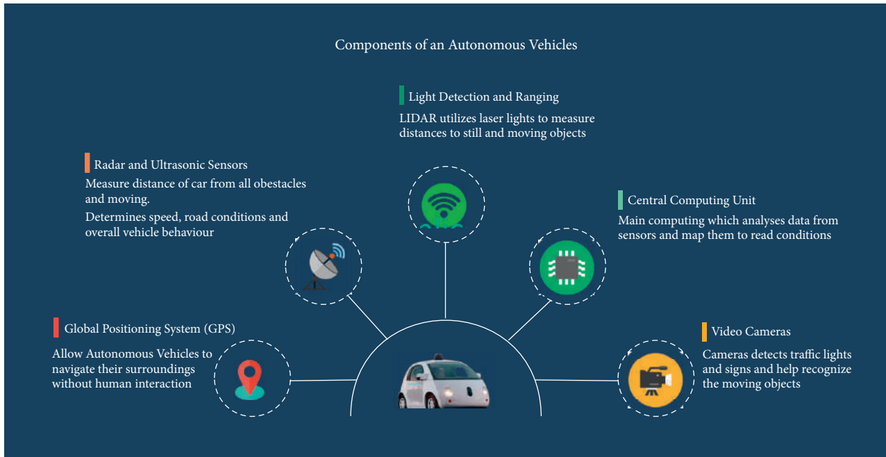
FIGURE 6: Components of autonomous vehicle.
